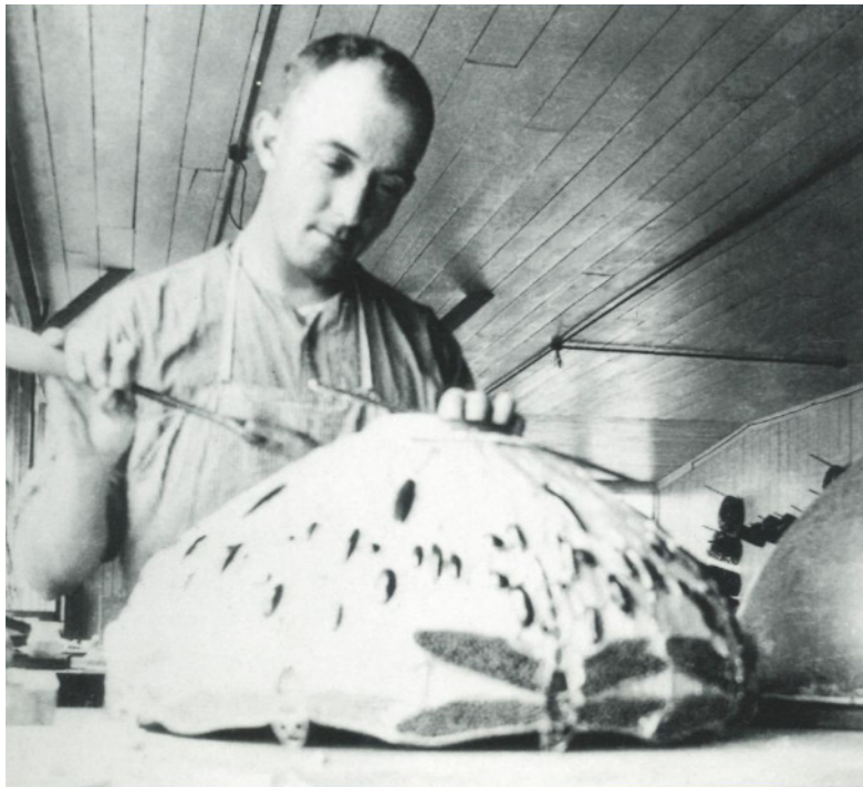
John Dikeman, Foreman of the Tiffany's Studio Lamp Department, applying a soldering iron to a 22-inch Dragonfly shade, 1915-20
